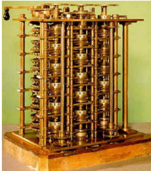
Fig S-1. Part of Babbage's Difference Engine.
